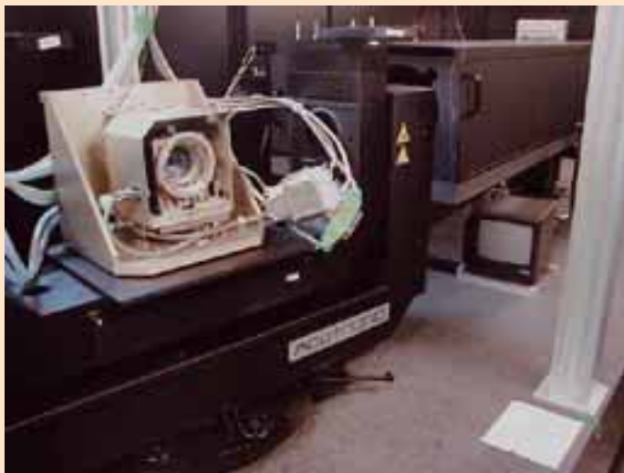
Sodern BCG16 star tracker test bench.
